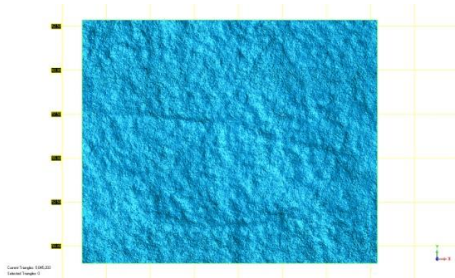
Photogrammetry 3D model (point cloud) Resolution 0.008 mm
